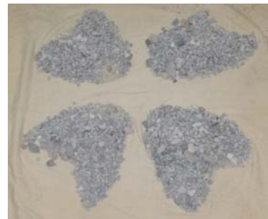
Remove two diagonally opposite quarters including fines.
