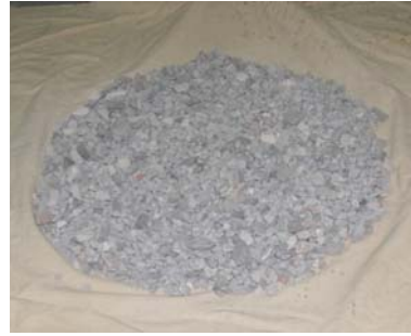
Flatten aggregate pile to a diameter 4 to 8 times the thickness.
