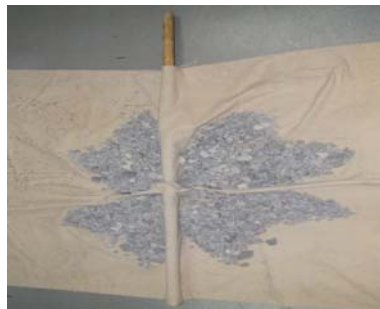
Divide the aggregate into four separate quarters using a shovel or stick.
